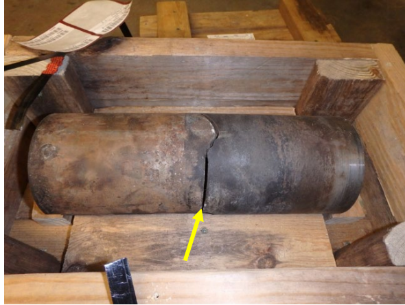
Figure 7. Fractured shaft that was packaged with the mating fracture surfaces touching (arrow).
