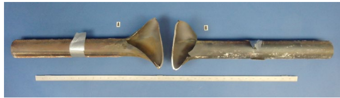
Figure 2. A boiler tube that was cut through the middle of the rupture prior to shipping.
