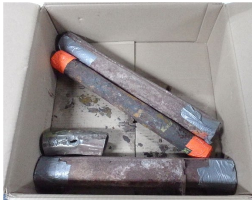
Figure 5. Box with four boiler tube sections and no packing material. Deposit can be seen that fell off of the tubes in the bottom of the box.
