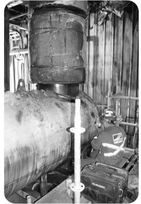
Acuren technician preparing the surface of equipment exposed to fire to obtain a "replica" for in-situ metallography
