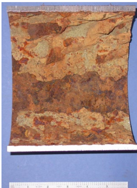
Figure 6. Internal surfaces of galvanized pipe from a hot, softened water line that was examined after two years in service. Pitting was significant on both sides of the pipe, but worse on the bottom of the pipe (shown here before and after cleaning).
