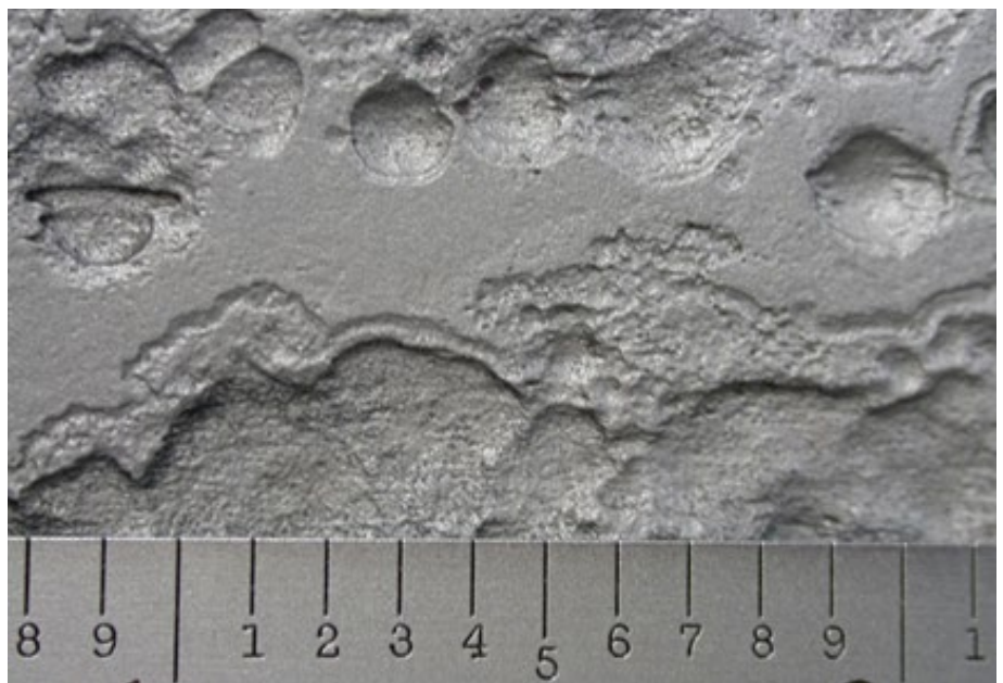
Figure 6. Internal surfaces of galvanized pipe from a hot, softened water line that was examined after two years in service. Pitting was significant on both sides of the pipe, but worse on the bottom of the pipe (shown here before and after cleaning).
