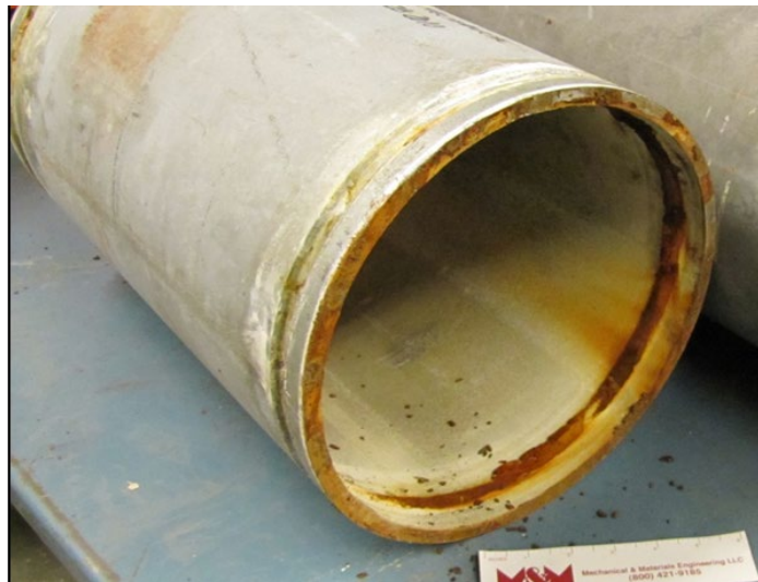
Figure 2. Corrosion along a rolled joint at the end of a galvanized pipe section.
