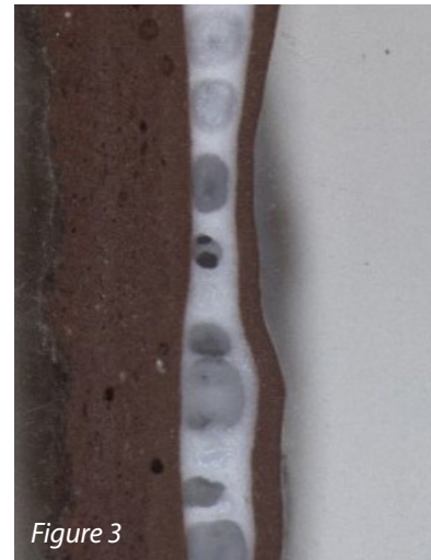
Figure 1: The paint blisters as they appeared on the siding. Figure 2: An opened blister reveals bubbles underneath the coating. Figure 3: A macrograph (~64x magnification) showing bubbles present throughout the primer layer.
