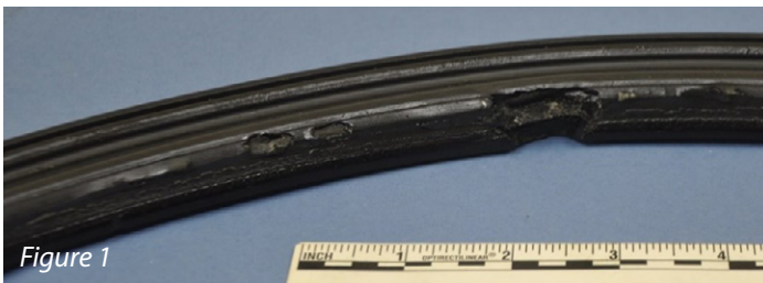
Figure 1: Photograph of the damaged propeller shaft seal. Figure 2: Propeller shaft lubricant samples were collected at various locations of the shaft. The lubricant sample on the left is a new reference sample. The samples show varying degrees of darkening and turbidity, which is indicative of oxidation and water intrusion.
