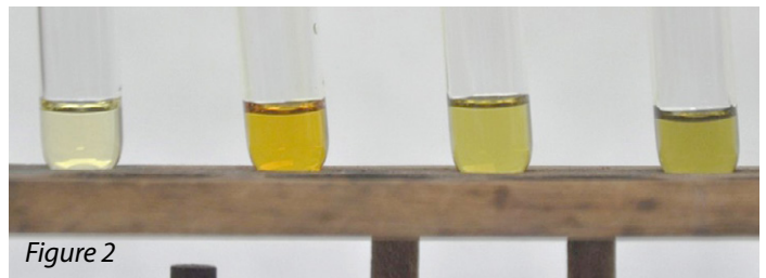
Figure 1: Photograph of the damaged propeller shaft seal. Figure 2: Propeller shaft lubricant samples were collected at various locations of the shaft. The lubricant sample on the left is a new reference sample. The samples show varying degrees of darkening and turbidity, which is indicative of oxidation and water intrusion.
