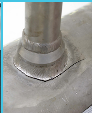
Fatigue crack at toe of weld
