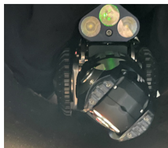
RVI inside piping using an explosion-proof robotic crawler
