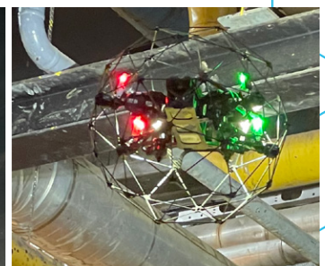
RVI of piping with collision-tolerant drone
