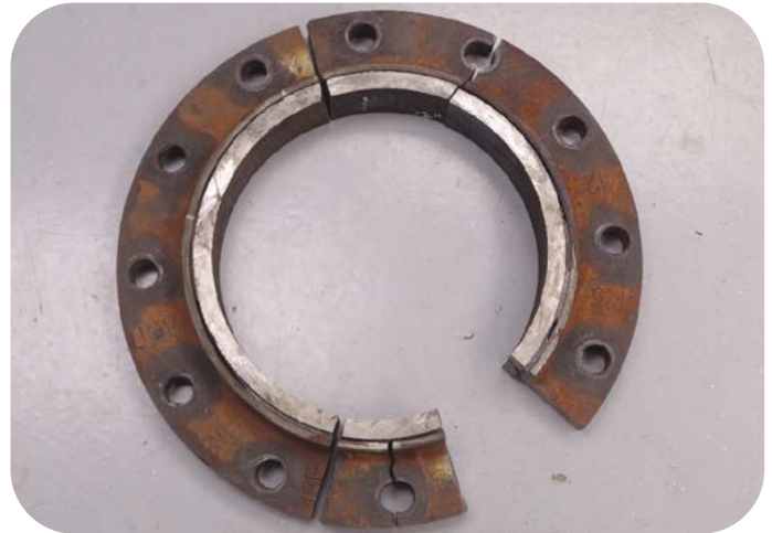
Image of failed flange after sectioning
