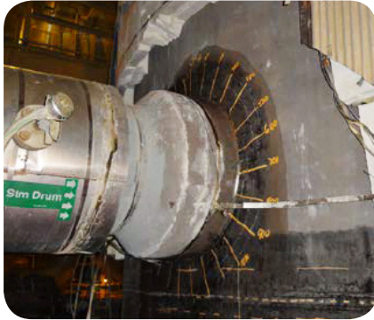
Transverse cracking detected at 550°F
